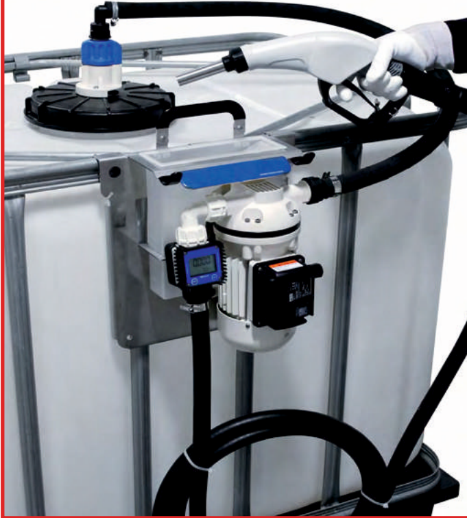
Ad-Blue Dispensing unit with electric pump 230v 32l/mn (7,04 gal/mn), meter and automatic nozzle. Suitable also with 12 v pump and for drums 208 l
